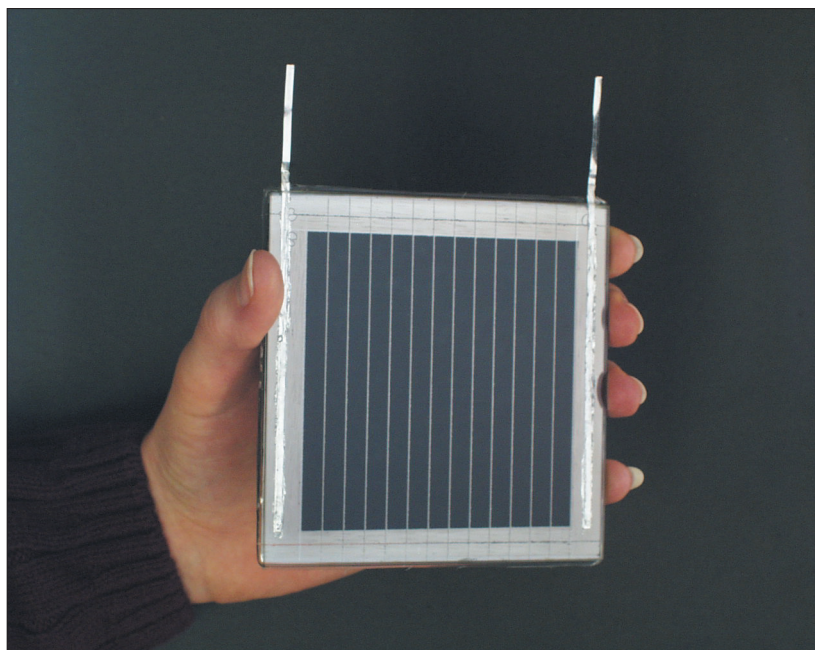
Fig.2: Encapsulated \text{CuInS}_2 module with 13 integrated series connected cells on a 10 \times 10 \text{ cm}^2 glass substrate
